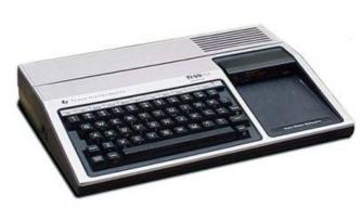
By today's standards, the TI-99/4A is a laughably under-powered machine. But with a 3MHz CPU, 16K of RAM, and display resolution of 32 characters/24 lines (text) and 192×256 16 colors (graphics), it was pretty capable as compared to other machines of the era.
