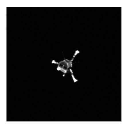
Philae was supposed to tether itself to the surface of the comet, but the tether harpoons did not fire. Because of the low gravity, the Philae lander bounced twice, eventually coming to rest against a cliff face. Its instrumentation was not damaged, but unfortunately its position kept it from receiving adequate sunlight for its solar panels.
